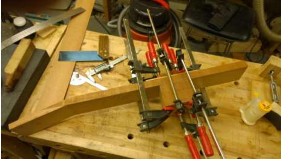
I used a router table to make a slot for a two way truss rod.
