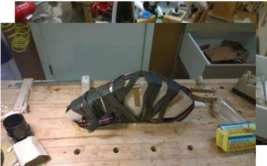
I used my hot pipe to bend all the strips to the two falcate brace shapes. I bend them at better than 2 times the width. After they are laminated I rip each to make the pair of falcate braces.
