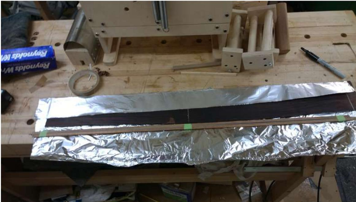
I use a Fox style bender named after Charles Fox, a luthier known for designing small shop guitar jigs. The wood is heated to about 300 F and bent into a mold.
