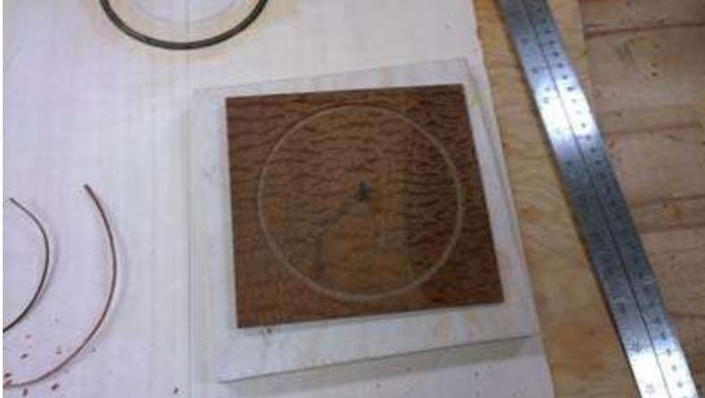
After first trying to cut the second ring I noticed that I needed to scrape the ring level so that the router will cut the next channel at the correct depth.
