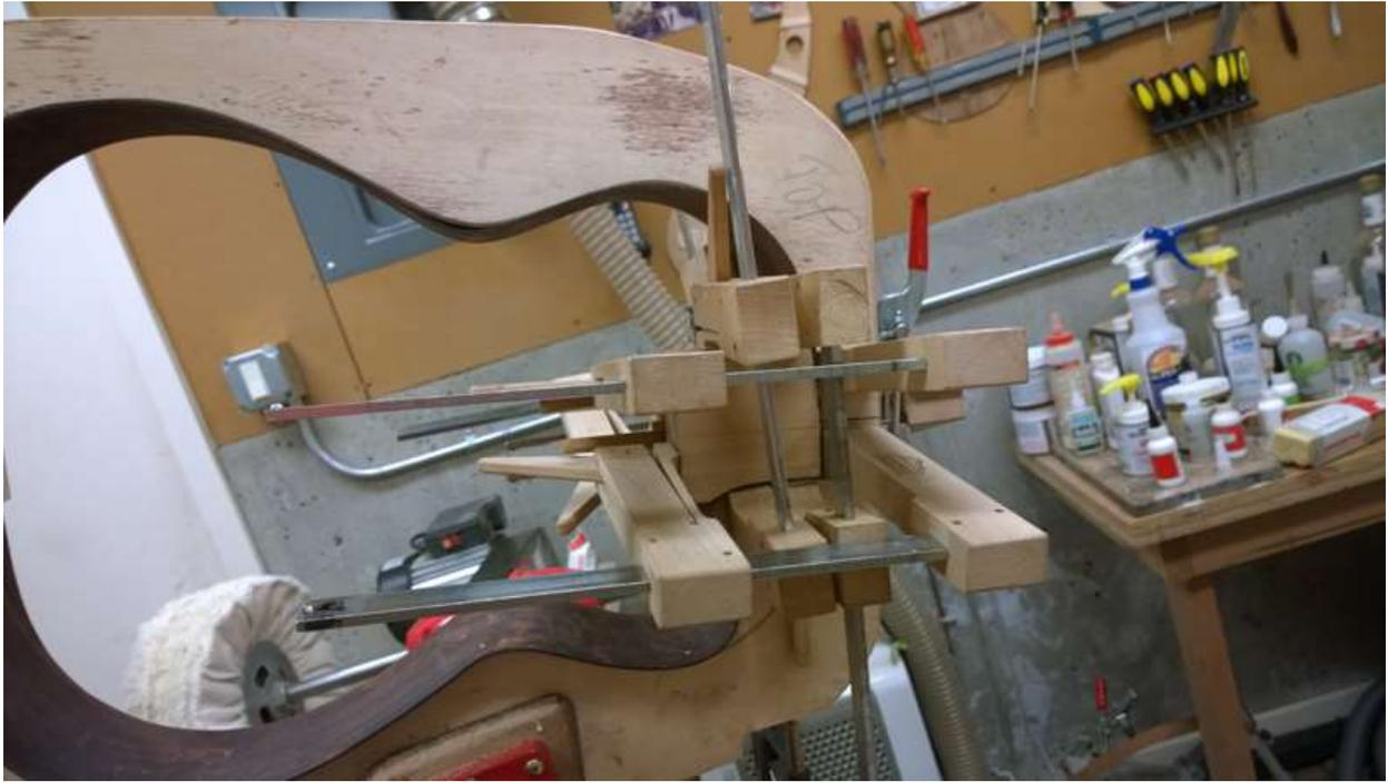
Here are the rims with both the heel block and a plywood tail block glued on. Not shown in the pictures, the back rims of this guitar were profiled with a 10' radius dish to give it a pretty significant curve. The top rims were profiled with a 32' radius dish. It curves the top and provides the start of the neck angle built into the rims.
