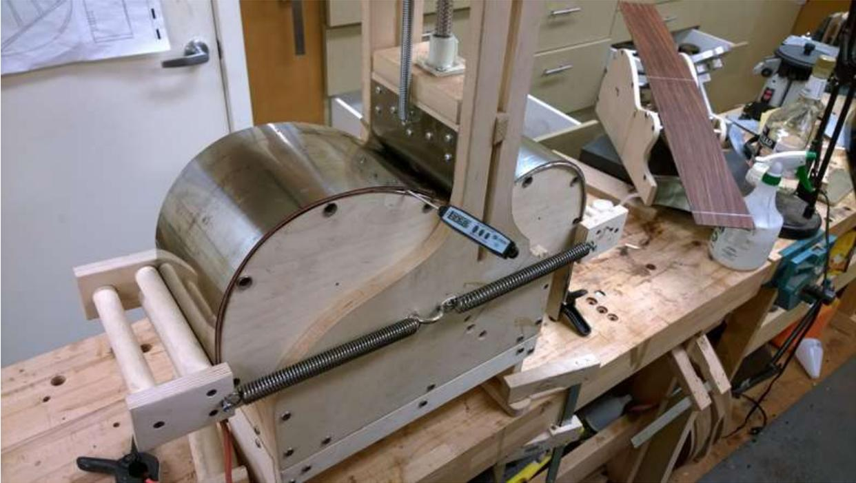
The Venetian cutaway that this guitar will have requires a very tight and difficult bend. To make the bend possible I first thinned the tightest part of the bend a quarter of a millimeter using a cabinet scraper. I also sprayed the side with Supersoft II a veneer conditioner. I use a separate mold and an extra press to make the Venetian cutaway bend.
