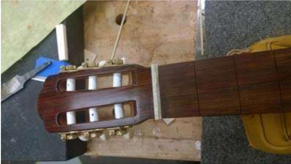
The Book has a table and tells how to make a table to calculate nut and saddle compensation based on scale length, strings and action. As I mentioned, I was able to use the example in the book. The table includes the active string length for each string. I used that measurement from the nut to mark out the saddle compensation.
