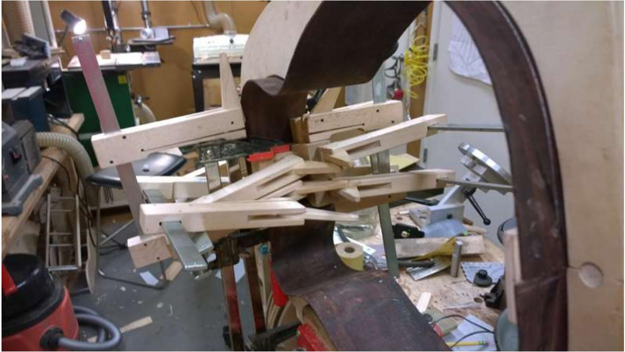
As shown a few clamps are required to get block properly glued to the sides.
