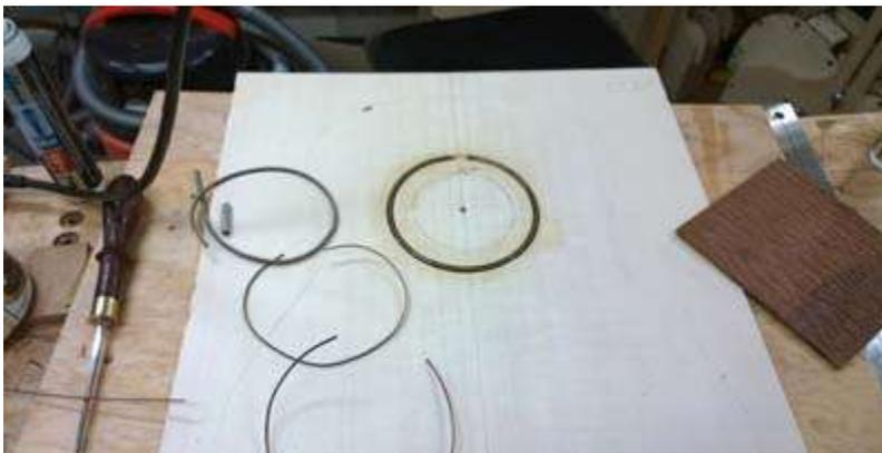
Before moving on to the next channel, the router base is set up perfectly to cut the outside of the wood rosette. I only cut to the depth that matches the thickness of the rosette channel. So without changing anything I cut to the outside line of the wood rosette. No measuring just negative space.
