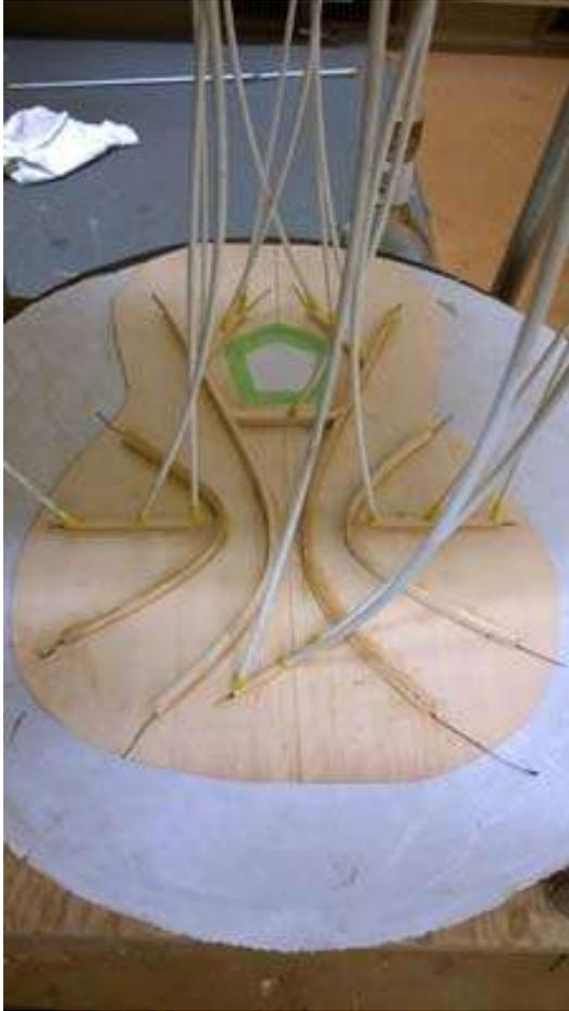
I was a bit more deliberate while epoxying on the braces and carbon fiber and overall I was less messy. Still have a ways to go in that regard.
