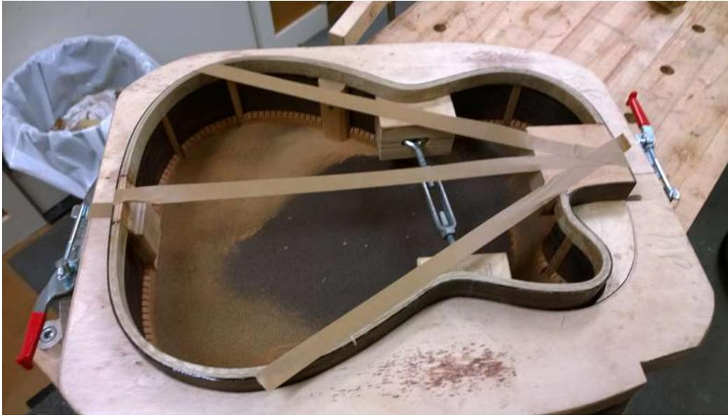
Here the rims are assembled and profiled.
