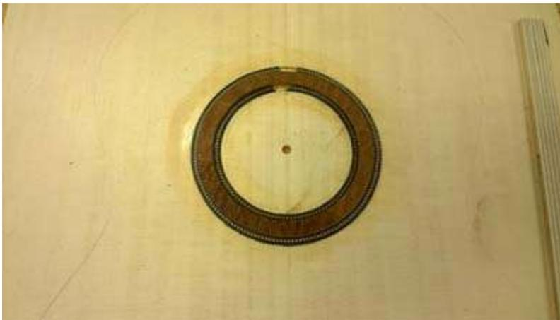
The ring snapped right in place. Not wanting to break it by pulling it out, and having previously sealed the inside of the channel with shellac, I flooded the rosette with thin CA glue.
