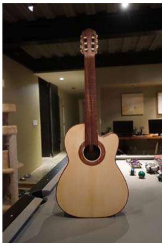
The finishing process takes a few weeks. I use zpoxy (a finishing epoxy) as a pore fill. Before filling the rosewood, working with rosewood and white purfling lines I mix a small amount of zpoxy up, dilute it with alcohol and seal the bindings and purflings. The stuff dries to tack within an hour or so. At that time I zpoxy the rest of the instrument.
