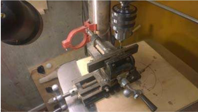
I mounted the blank (actually the second attempt) in my routing jig. In the first attempt I relied only on double stick tape and it did not stick. I cut that spoiled bridge diagonally and made the wedges that you can see in the photo.
