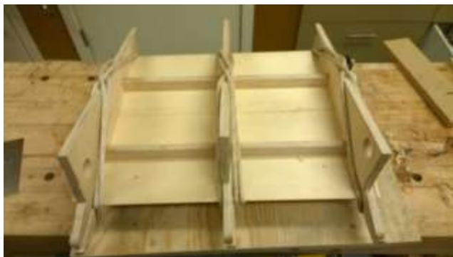
I used a plane and a shooting board to make a perfectly flat edge on the two pieces of spruce that will make the soundboard of the guitar. The gluing jig is based on an old Egyptian design using ropes and wedges to apply a joining force while keeping the plates flat.
