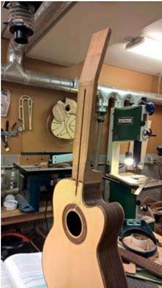
I cut close to the final taper of the neck in the heel portion. This allowed me to fit the neck to the guitar and check the neck angle before I routed the pocket in the top for the fretboard extension tenon.
