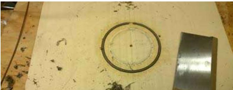
My stack is just a touch wider than my bit so I take a few passes and sneak up on the correct width. I make sure that any needed passes are going into the wood rosette area so that the router base is set to cut the inside of the wood rosette. Later when I run the back of the rosette blank through the drum sander a perfect sized ring should drop out.
