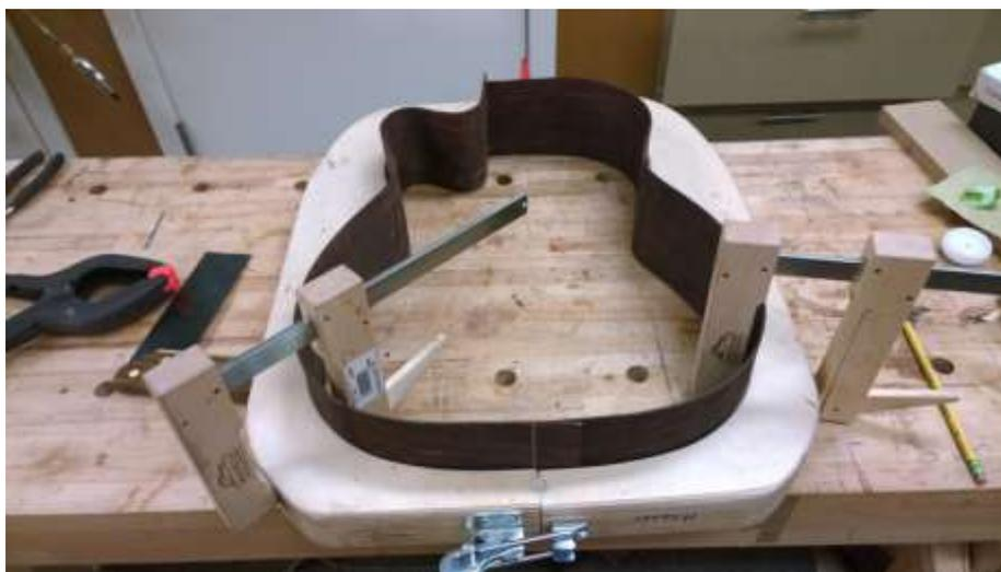
This guitar will have a bolt on bolt off neck. The heel block is larger than most as the neck will join the body in a mortise and tenon between the neck and the rims and another mortise and tenon under the fretboard extension. The block also needs to be shaped to support the cutaway side.
