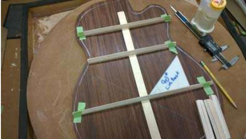
I cut channels in in the back center strip with a scalpel and chisel and rechecked the layout of the radial braces. I used a home built vacuum box to glue down all of the braces.
