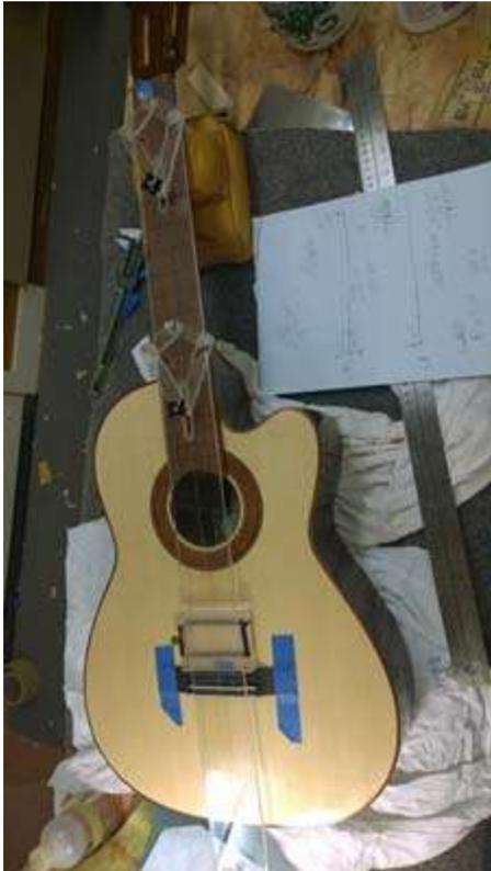
I set the fret board nut location to have a nut compensation as well as saddle compensation. I really spent a lot of time calculating and triple checking the location of the saddle. I did all of the measurements from the first slot as the fret board is about 3 mm short of the zero slot location. After it was taped in place I also checked the location against my other falcate classical (I could have thought about this first) and I had located it exactly in the same location.
