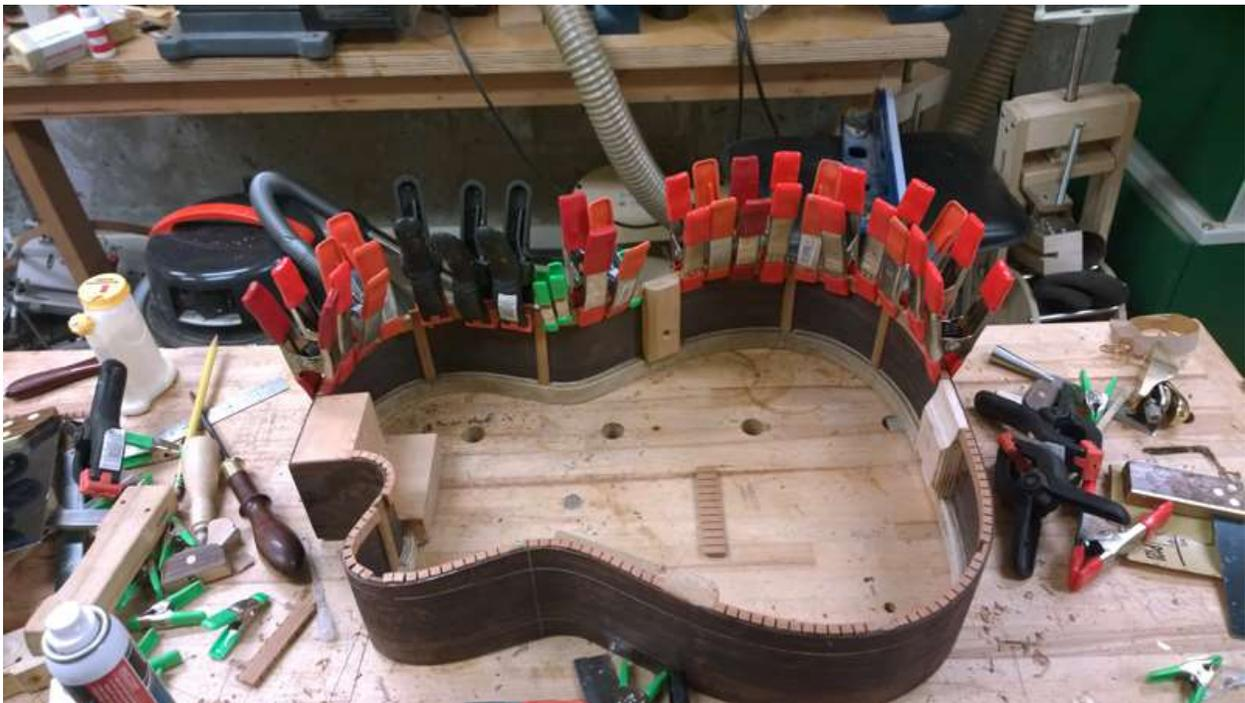
With both sets of linings installed I used the previously described 10' and 32' radius sanding disks to put the final profile on the rims. The tape in the picture is just there to stop me from sanding the top on the back's radius disk.
