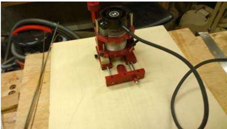
Instead of routing out the whole channel, I decided to make it on the sound board one section at a time. That way I can create tight channels for the rope binding and the EIR\B strips
