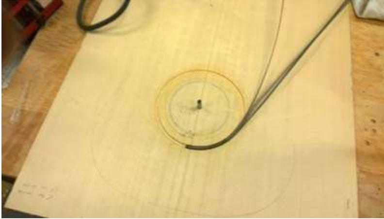
Ultimately I pulled out my bending pipe, bent everything close to the correct shape and found it easy to inlay the stack. I sealed the channel with shellac and I pushed the stack in place and flooded it with thin CA glue.
