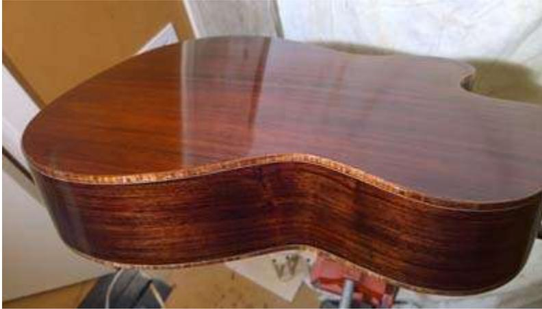
Before finishing the top I looked for glue on the top with a black light. Yup I had some smears in the center and some along the bindings. You can see the bright spot in the lower bout especially along the edges. This is after I thought I had the top clean.
