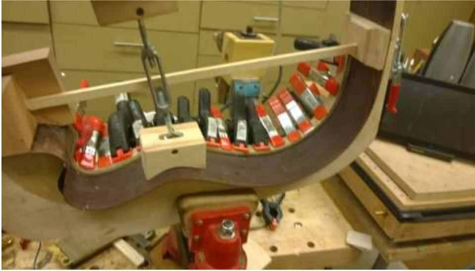
To finish the rims I fabricated and installed a couple of side mass mounts and some rim reinforcement strips. The side mass mounts allow one to add a heavy plate to the rims to lower the tops resonance if required during final setup. Here I am gluing on some standard kerfed linings to the rims for the back.
