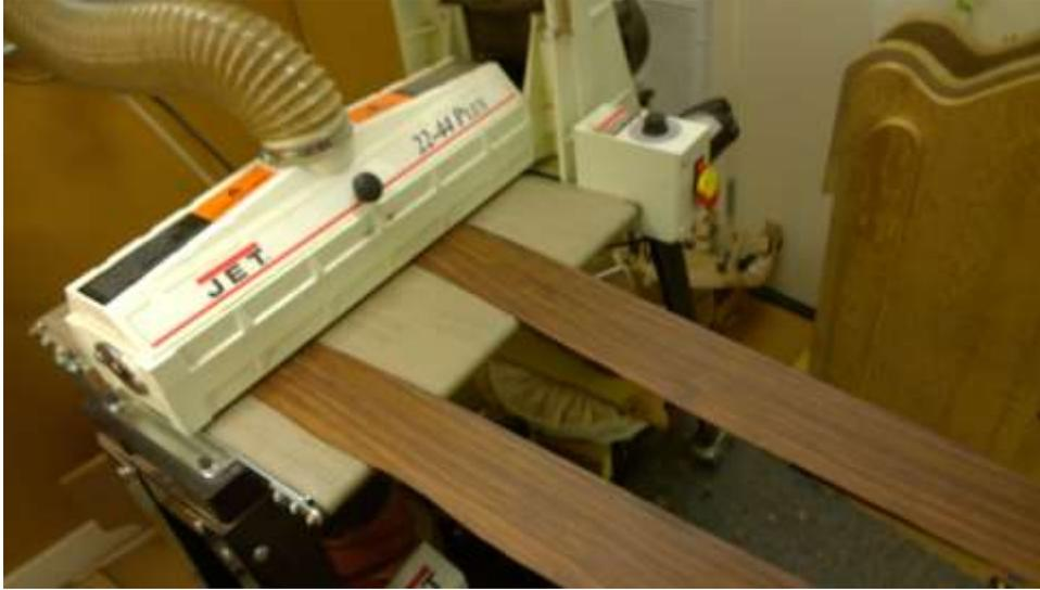
The sides are profiled using a template I made the last time I made this style of guitar and thicknessed to about 2 mm using a drum sander. Preparing to bend I also include a set of bindings with each side that I will use to trim the guitar body.
