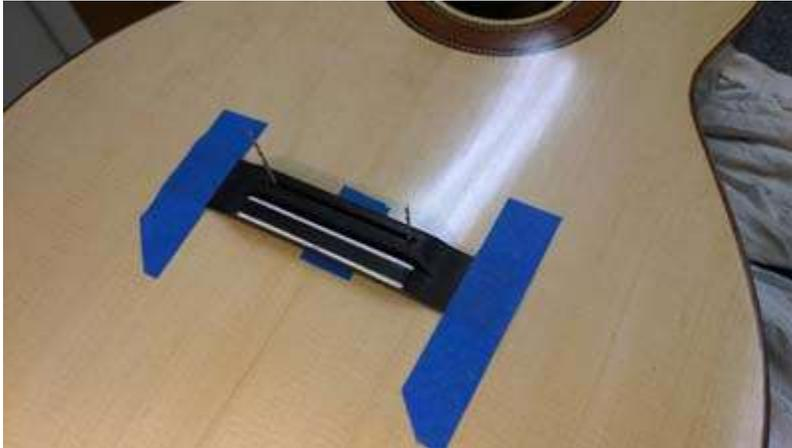
With the bridge in place using a new scalpel blade I carefully scored the finish and used a utility blade (actually three by the time I finished) to scrape the shellac under the bride.
