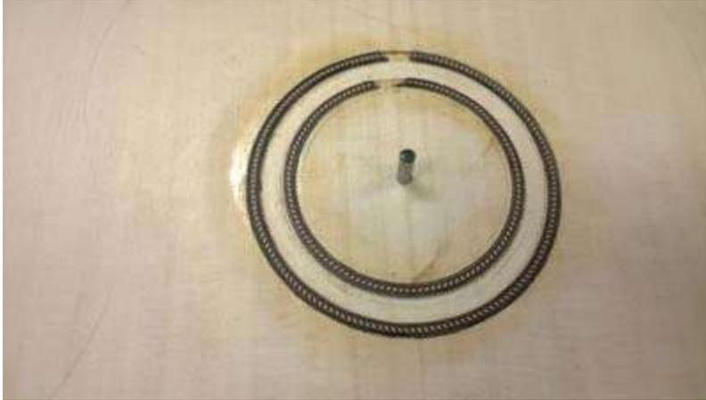
I routed the inside of the rosette channel sneaking up on the black fiber. This is where the Bishop Cochran base shines. I have gotten to where I can move the bit in .01 mm increments.
