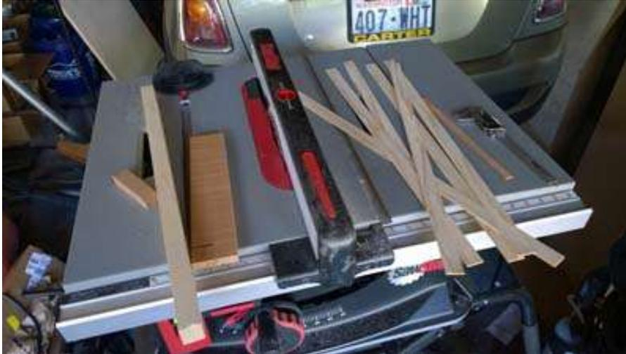
I used my table saw to rip a whole bunch of 1.7 mm strips that I used to make the laminated falcate braces
