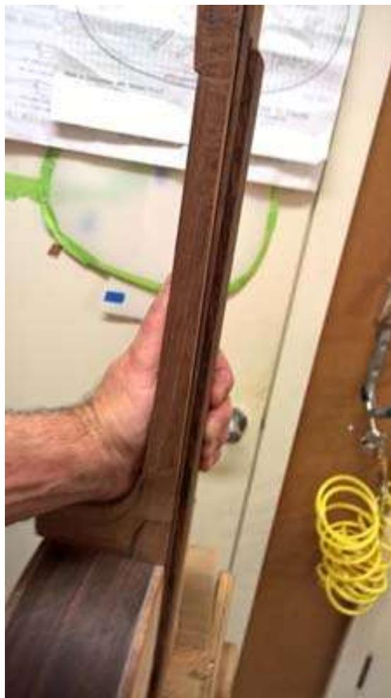
Note how the mahogany glued to the fret board is sloped 4mm to 0 mm to give fret board a negative slope
