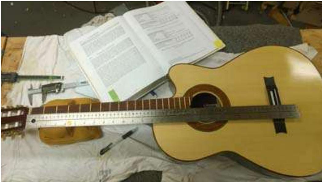
The guitar is complete and it sounds pretty good. Since I completed the guitar I made a new nut to allow for some more spacing on the edges. This of course narrowed the distance between the strings at the nut. Here is a final set of photos
